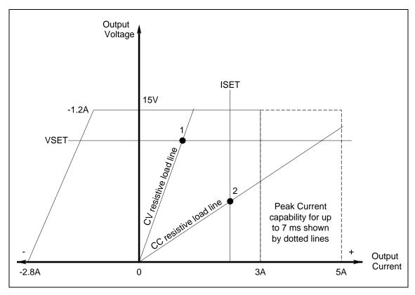
Figure 2-1. Dc Source Output 1 Characteristic
